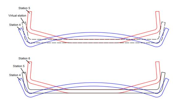
**Top picture:** Virtual pass. After unbending the radius, complete flat area elements are joined together and the overbend of the complete base is created.
